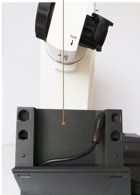
Control panel support
