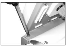
→ Use Phillips screw driver to remove both screws at the fixing plate of the controller and remove controller.
