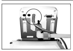
➡ Remove control cable at the rear side of the controller. Do not cant when removing plug connection!
