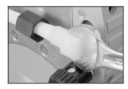
→ Use open ended wrench (w/f 14) to reconnect hose to elbow fitting.
