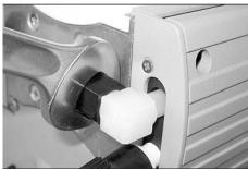
■ Use open-ended wrench (w/f 17) to loosen the union nut at the hose connection next to the gas ballast.
