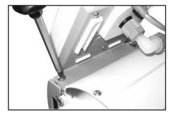
Unscrew both Phillips screws at the fixing plate of the controller
