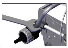
■ Use open-ended wrench (w/f 17) to loosen the union nut at the hose connection next to the inlet and remove hose.
