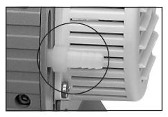
■ Unscrew the hose nozzle at the outlet of the pump using an open-ended wrench.
