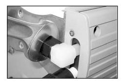
➡ Tighten union nut first by hand and then tighten one full turn using open ended wrench.
