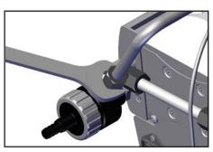
➤ Connect hose to the connection at the inlet of the pump. Tighten union nut first by hand and then tighten one full turn using open ended wrench.
