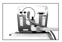
Connect control cable to the rear side of the controller. Do not cant when assembling connection!
