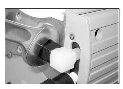
■ Use open-ended wrench (w/f 17) to loosen the union nut at the hose connection next to the gas ballast.
