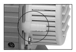
■ Unscrew the hose nozzle at the outlet of the pump using an open-ended wrench.
