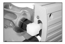
→ Tighten union nut first by hand and then tighten one full turn using open ended wrench.
