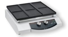
Fig. 2: Example of a vibration shaker for multi-well plates: Titramax 1000 by Heidolph Instruments
