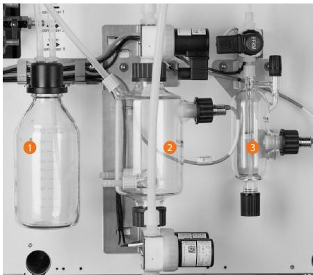
Use of the automatic Hei-VOLUME Distimatic Pro module with a rotary evaporator Hei-VAP Industrial requires a special set of glassware consisting of a Woulff bottle [1], a collector vessel [2] and an educt sensor vessel [3].
