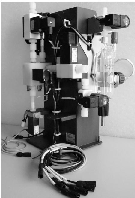
A Hei-VOLUME Distimatic Pro & Hei-VAP Expert/Ultimate system consists of pre-assembled assemblies (condenser, valve matrix).
