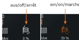
The operating behavior is defined by the process parameters of the selected mode (automatic switching on, on-period/pause time in percent). Example: Period 100 %, defined heating tape on-period 30 %, pause time 70 %, for a 100-second cycle, equates to an on-period of 30 seconds per cycle.
