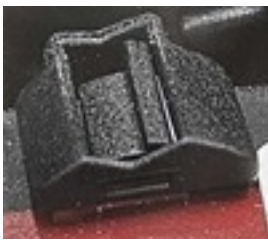
Black field: Direction of rotation correct
