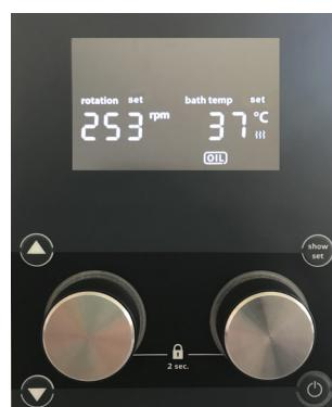
The value selected in each case is adopted as the new setpoint when the controller is pressed (start the function).
